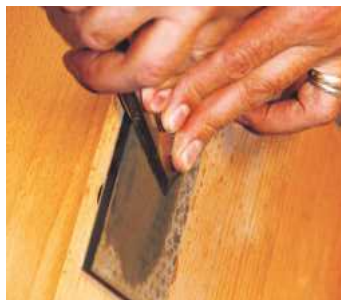
▲ Smaller credit card hones work well for touching up router cutters
